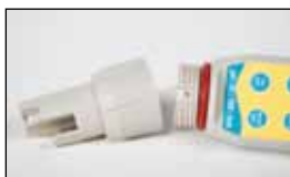
Sensor includes both pH and conductivity/TDS/salt probes.
