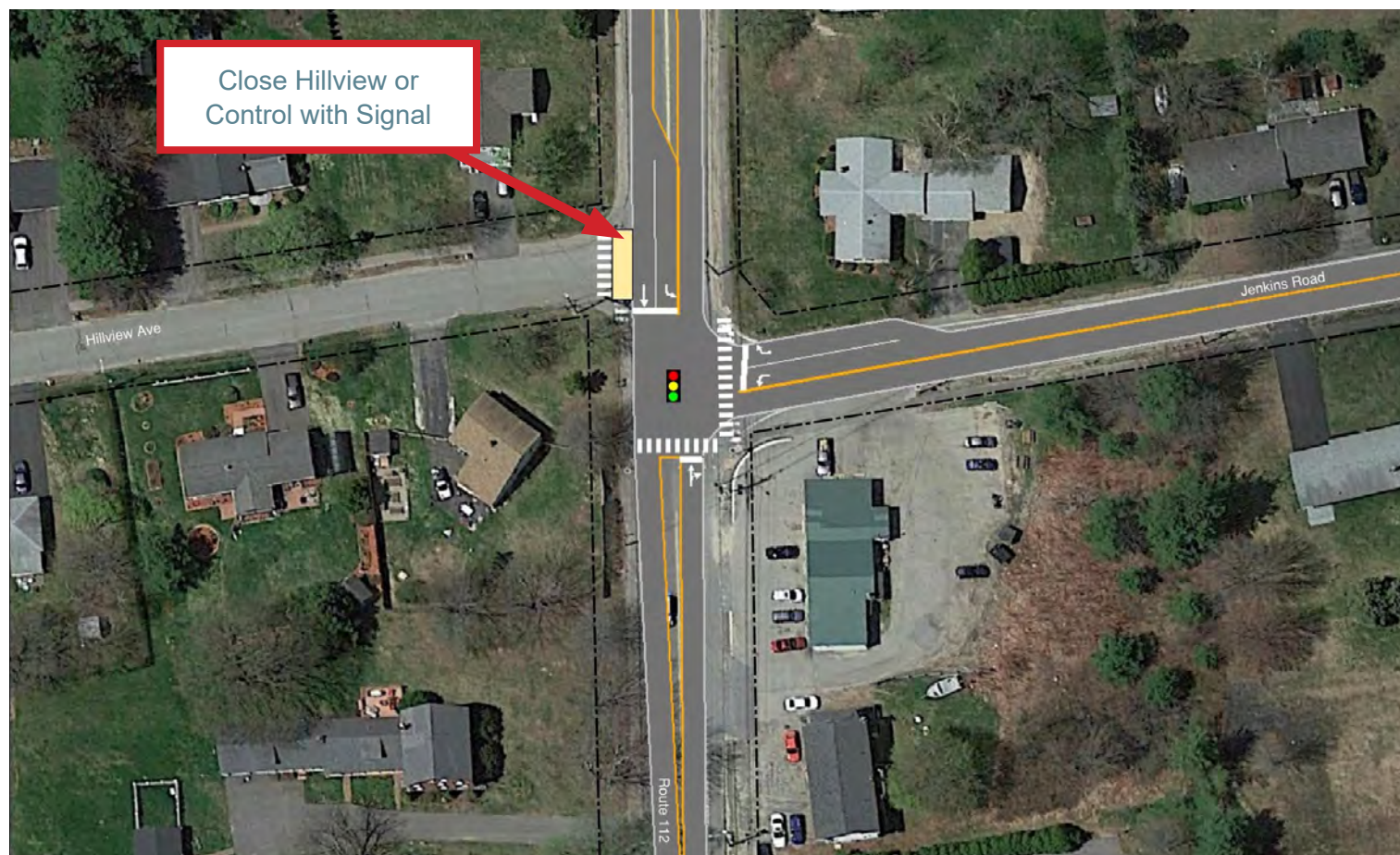
Figure 11.1 Route 112/Jenkins Road Short-term Improvements
